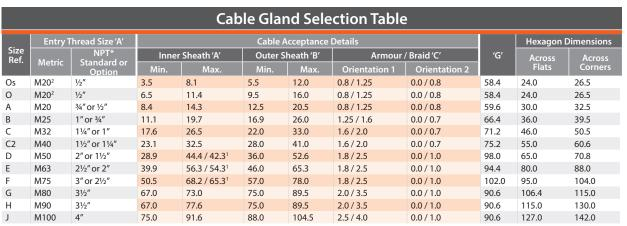
'F' - Os-F size metric entry threads are 1.5mm pitch as standard, 15mm length of thread. For G size glands and above, a 2mm pitch is supplied as standard, 20mm length of thread (1.5mm pitch with 15mm length of thread can be supplied) please specify when ordering. G size and above are available in the 501/453/RAC design style. All dimensions in millimetres (except \* where dimensions are in inches).
