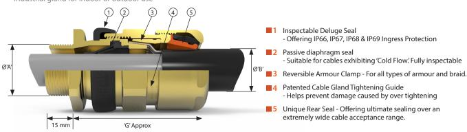
The industrial 153/Universal Cable Gland is robust and for use with single wire armour 'W', wire braid 'X', steel tape armour 'Z', elastomer and plastic insulated cables. For particular use with cables that exhibit 'Cold Flow' characteristics.
