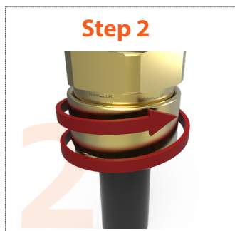
Step 2 Tighten backnut until a seal is formed onto the cable, then tighten one further turn
